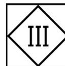
**Class III** – This type of equipment is supplied from what is known as a SELV (Separated Extra Low Voltage) source which will not exceed 50V a.c. Generally Class III equipment will not require PAT testing. Mobile phones and Laptops are examples of Class III equipment. One thing to note with Class III equipment is that although the equipment itself may not require PAT testing, its associated charging equipment may.
